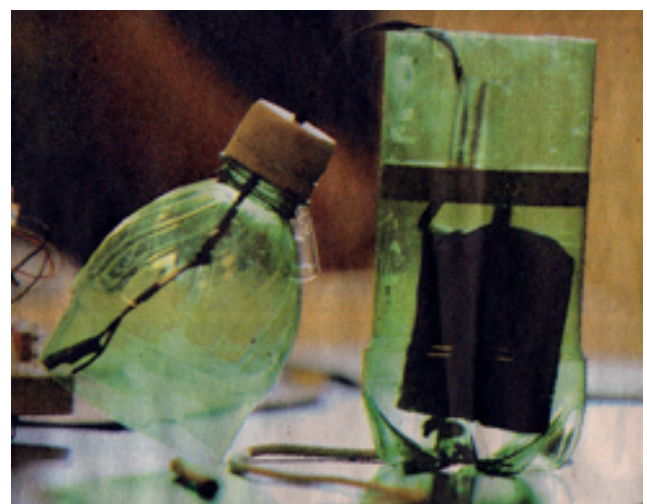
The flashlight is made from items available in those countries: a soda bottle, wood, wire and a battery.
